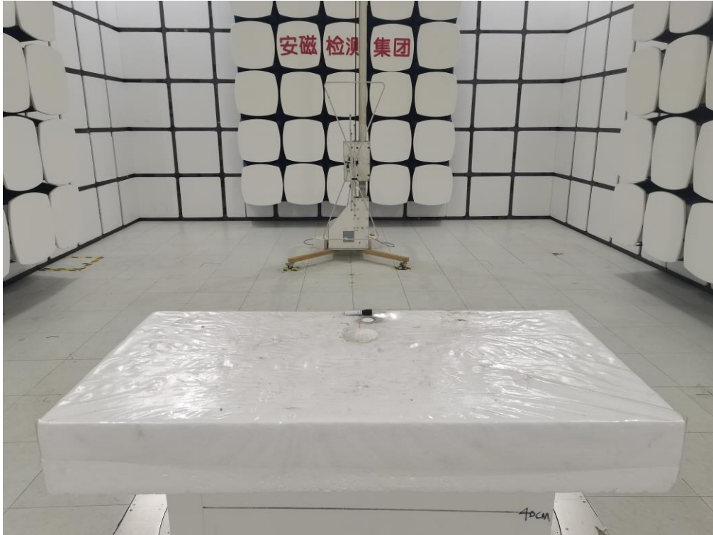
Radiated Measurement Photo
